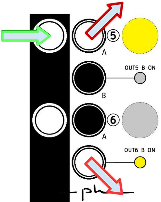
The incoming signal on channel 5 is routed to output 5A (and inactive, "muted" to 5B) because the illuminated push button is in the pressed position (LED on). The "OUT5 B ON" LED is off.
